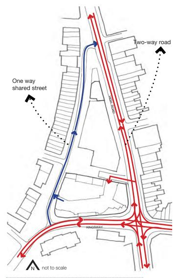
Figure 25: Re-routing of Ballards Lane through traffic
