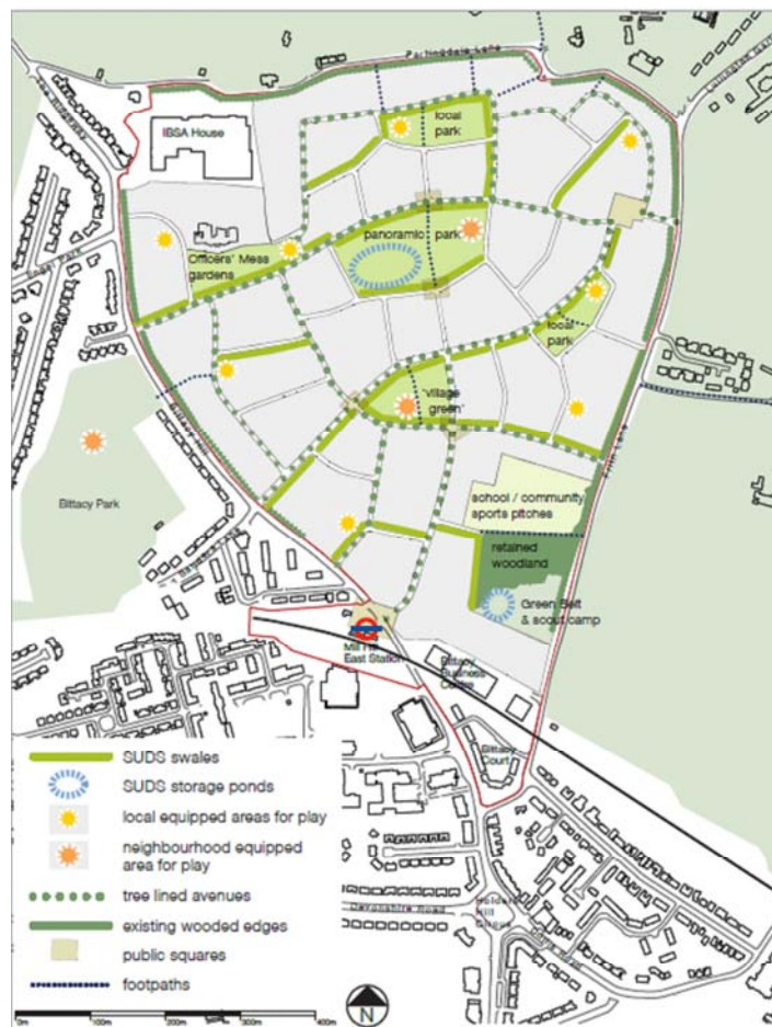
Map 2: Open Space and Sustainable Urban Drainage Masterplan for Mill Hill East AAP
