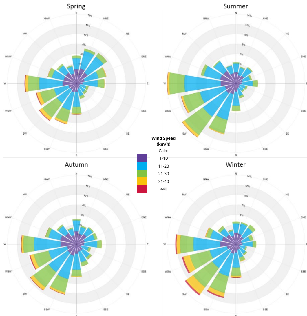
Figure 3: Seasonal Wind Roses for London Heathrow (in km/hr) (Radial axis indicates the percentage of time the stated wind speed is exceeded)
