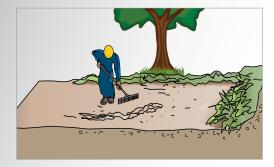
Install TRP4000 geotextile. Overlaps by minimum 300 mm.
