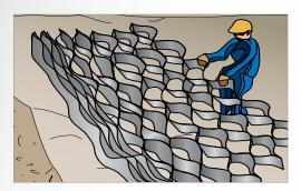
4 Connect GEOWEB<sup>®</sup> sections with ATRA<sup>®</sup> keys.
